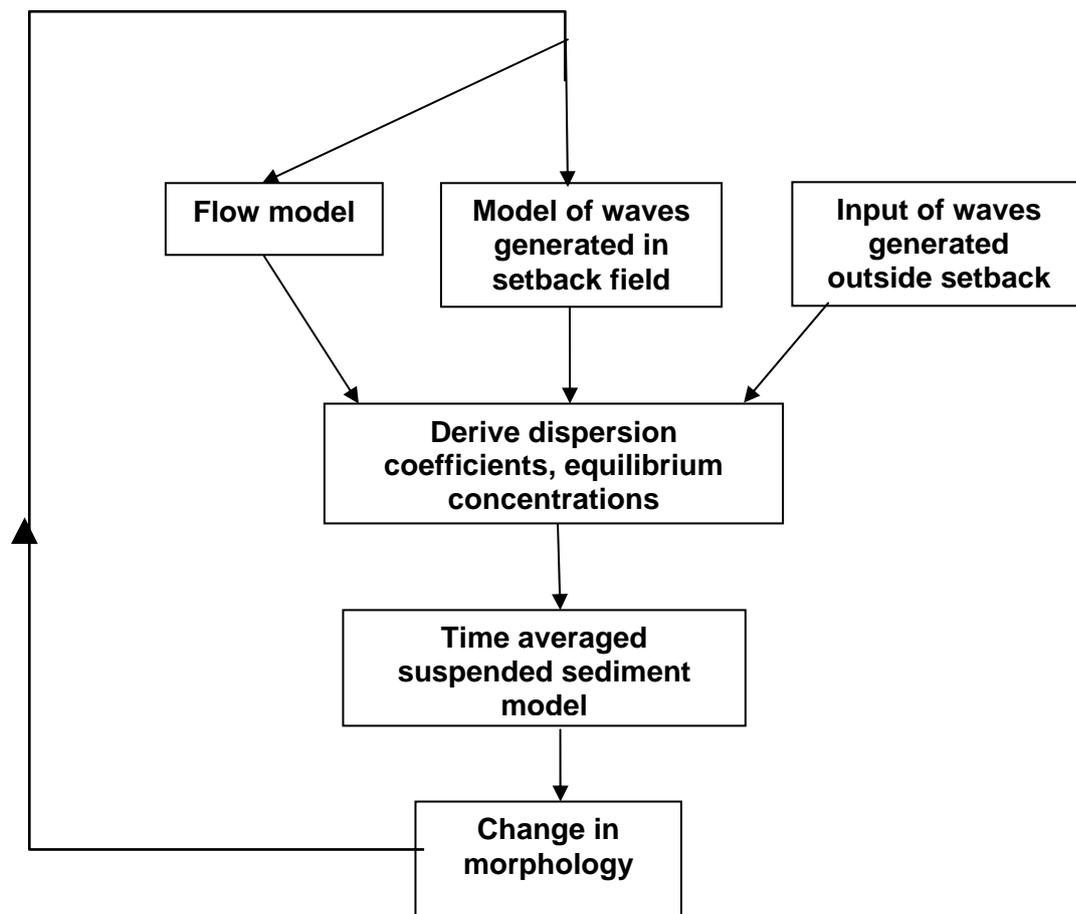
Figure 1. Basic structure of morphological Realignment model
