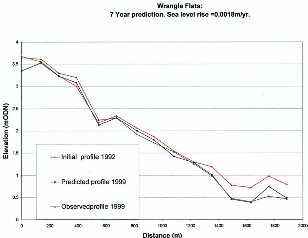
**Figure 7. Hindcast prediction of intertidal response at Wrangle Flats, the Wash, using Mudpack model (Pethick, 2002)**
